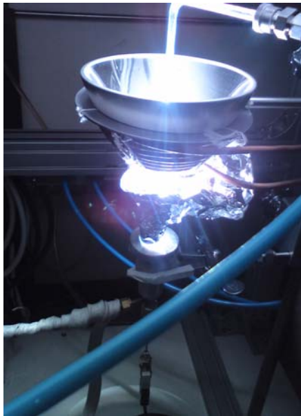
Fig. 3.4.15 Photograph of solar reactor experiment on CeO 2 coated SiC foam(left), hydrogen production amounts of CeO 2 /SiC foam in parabolic solar reactor system(right).
