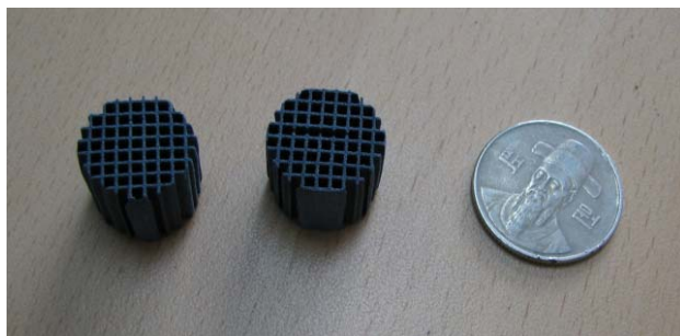
Fig. 3.4.10 Photograph of SiC honeycomb(200 CPSI)
