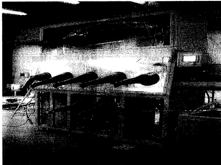
Fig. 83. Glove box for manufacturing the metal hydride hydrogen storage tank.
