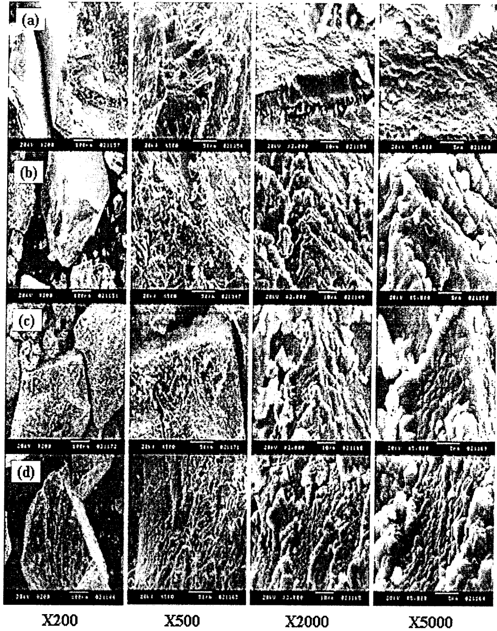
그림 2-2. SEM images of xerogel aged at different conditions at Si:P=5:5. (a) 70°C, 1 day, (b) 70°C, 5 day, (c) 90°C, 1 day, (d) 90°C, 5 day.
