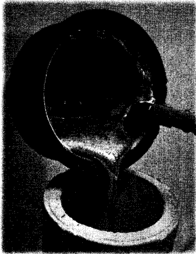
Fig. 3.2.3.3 The melting sample of the aluminum with flux A or D(5wt%)
