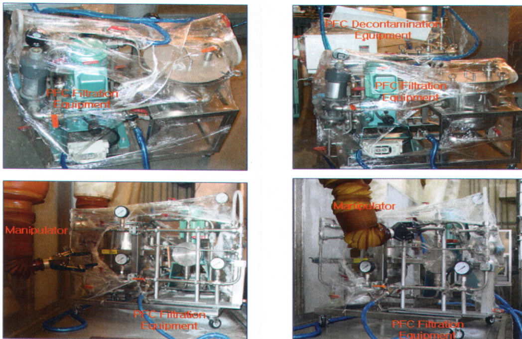
Fig. 3.1.4.81 Demonstration experiment of the improved PFC filtration equipment
