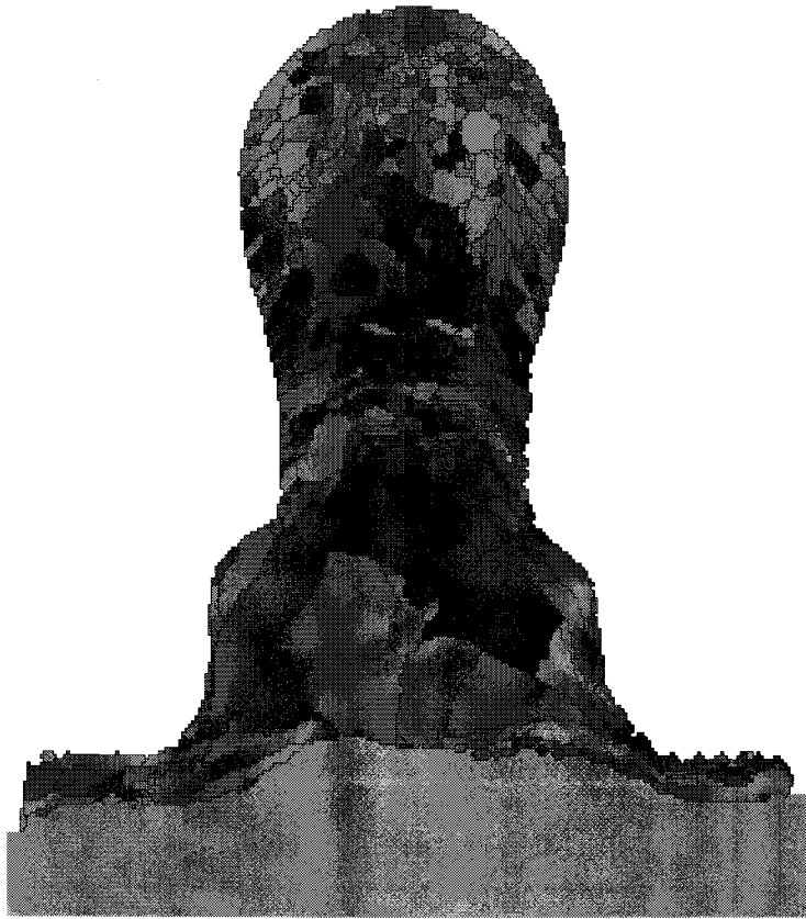
Fig. 3.4.2-1 Orientation maps of Gold Bonding Wire produced by M Electronics ( Measured by SNU Texture Control Lab. )
