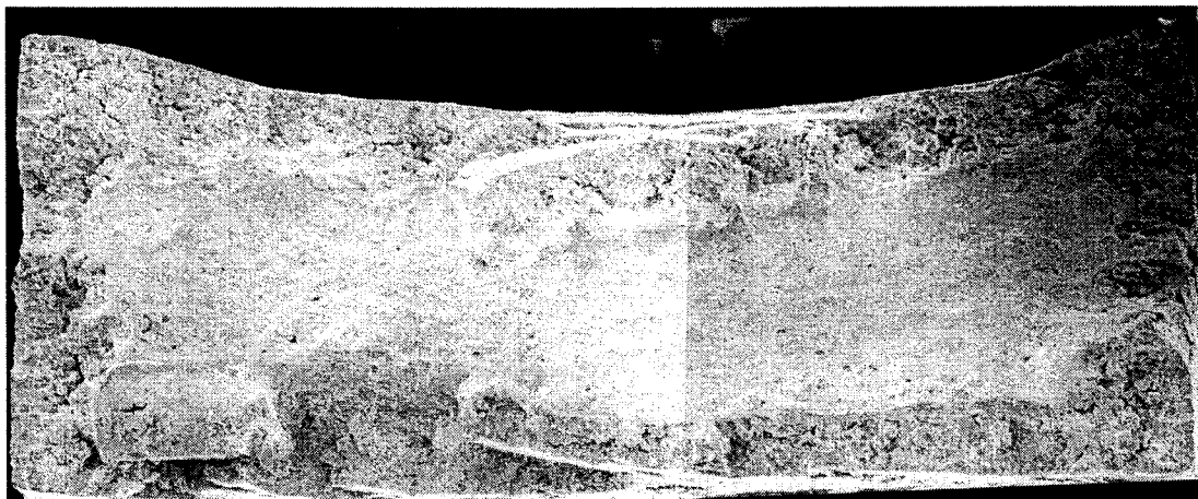
Fig. 3-2-8 SEM micrograph of Alloy 600 MA after SSRT in water containing 1000 ppm Pb at 300°C, pH 10, strain rate of 2 \times 10^{-7} \text{ sec}^{-1} , potential of -650 mV vs Ag/AgCl.
