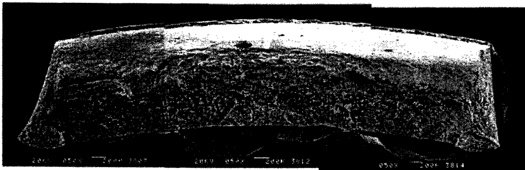
Hp72, 5 \times 10^{-7} /s, 50ppb ZnO, C, shoulder released, 45%
