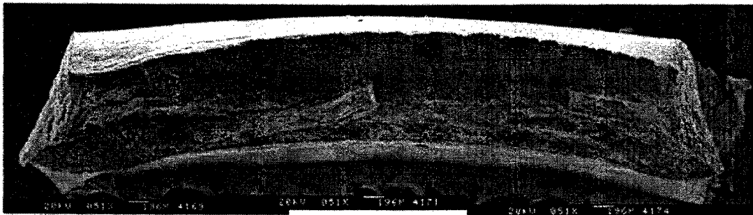
Hp72, 5 \times 10^{-7} /s, 50ppb ZnO, C, shoulder released, 45%
