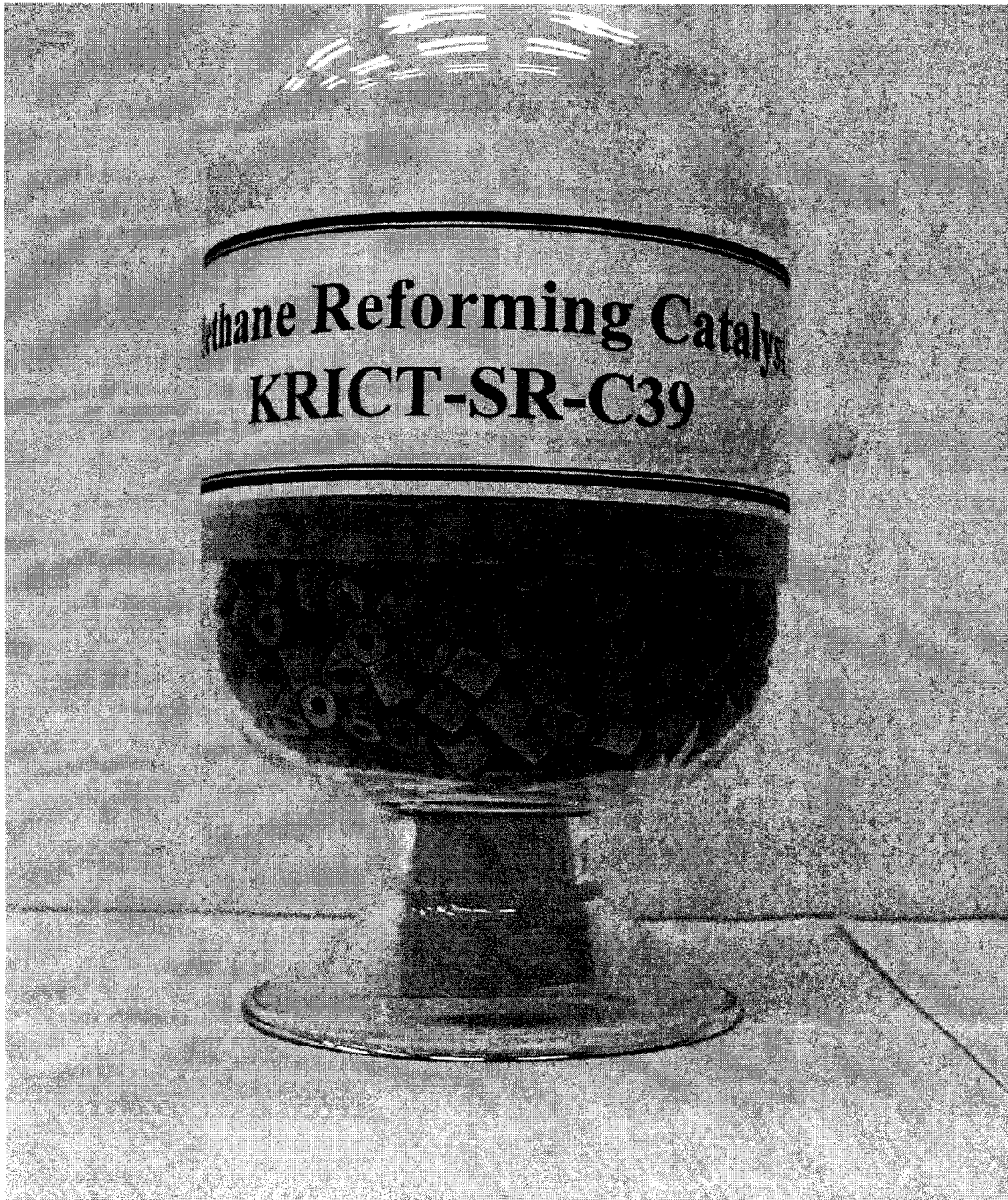
Figure 3.1.12. Reforming Catalyst (Modified Ni/Ce-ZrO 2 , Manufactured by KRICT).
