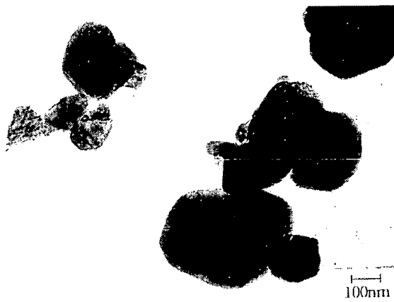
Fig. 5. TEM Microstructure of W-Cu base oxide powder
