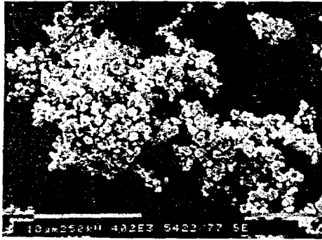
(a) 700°C 4hrs reduction powders.
