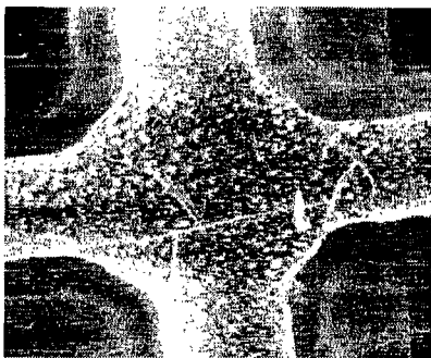
FIG. 3.F.5 LFM image of an imprinted APS pattern (focussed at a single intersection, A=10, B=20, and C=120, all in \mu\text{m} ).
