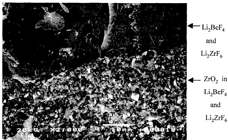
Fig. 5-7. SEM photograph of the LiF-BeF 2 -ZrF 4 salt and ZrO 2 formed by pyrohydrolysis.
