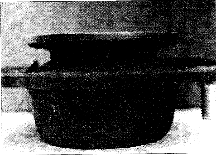
Fig. 5.33 Typical example for fatigue failure of rubber part
