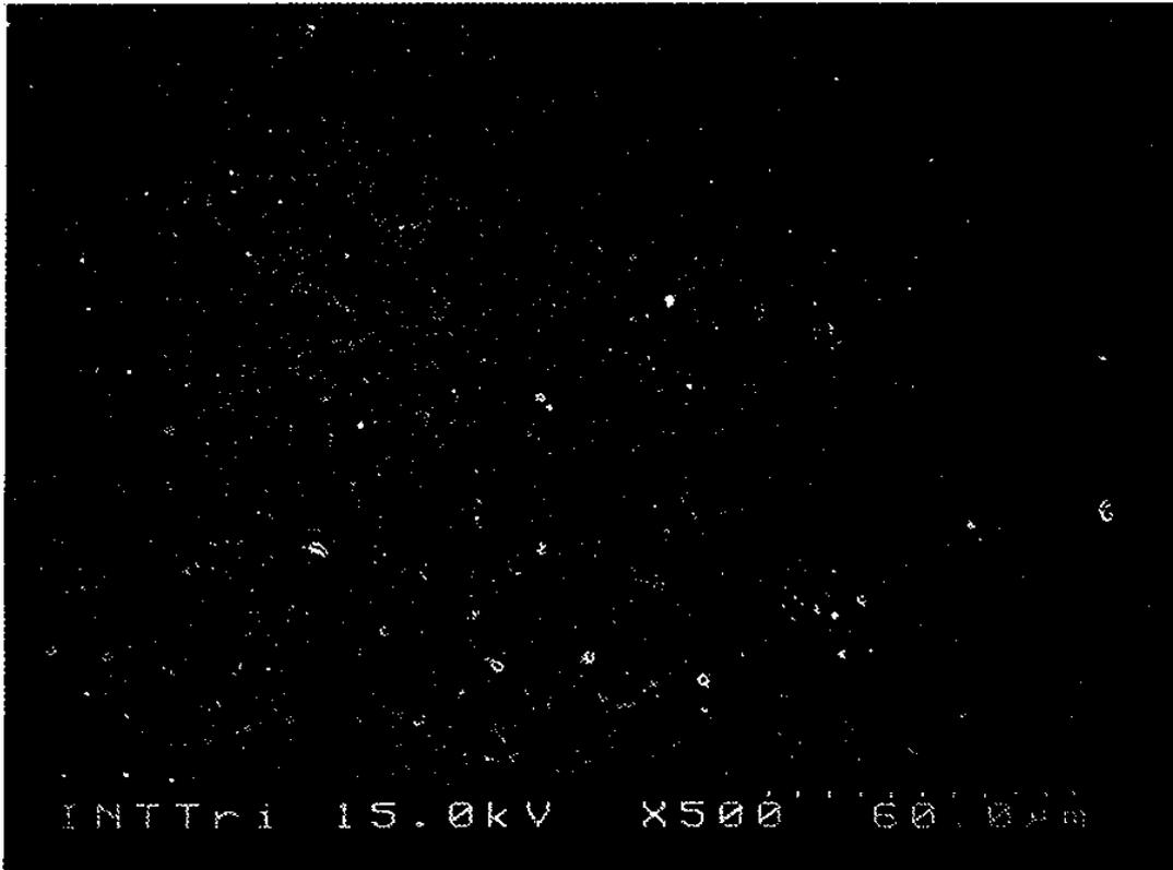
Fig. 20. SEM micrographs of polished and etched surface of L4 system showing fine microstructure of surface layer and coarse microstructure of inner layer.
