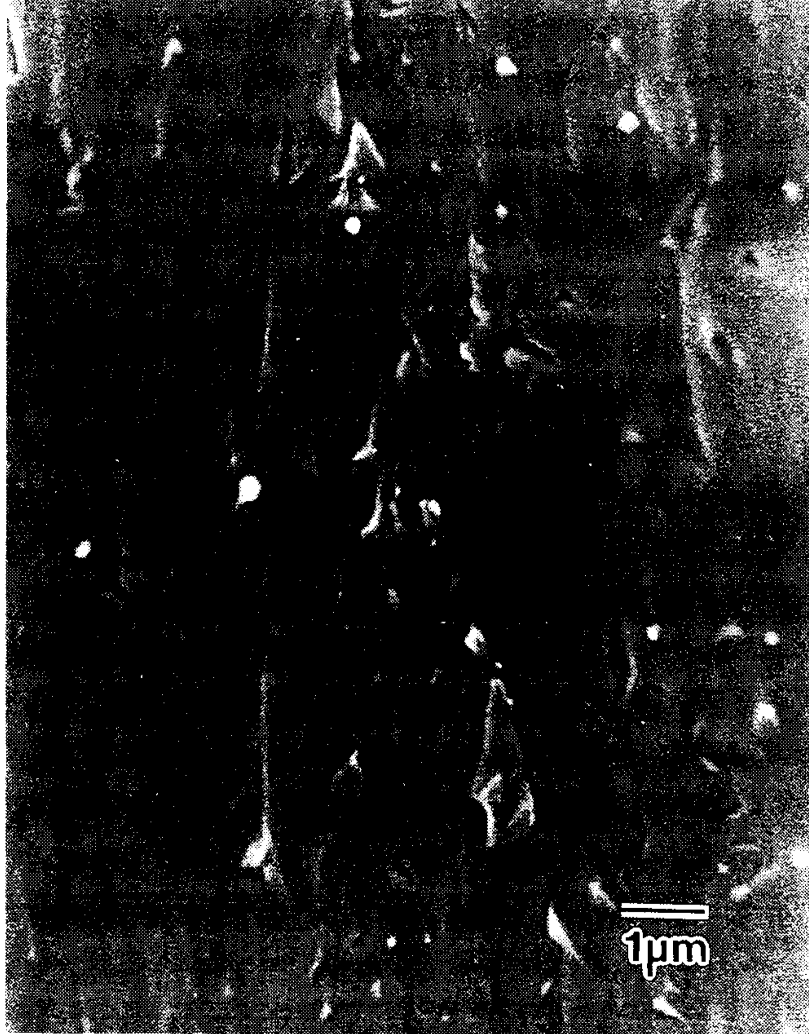
Fig.6. Scanning electron micrograph of the fracture surface of MDI/BD copolymer modified epoxy:
