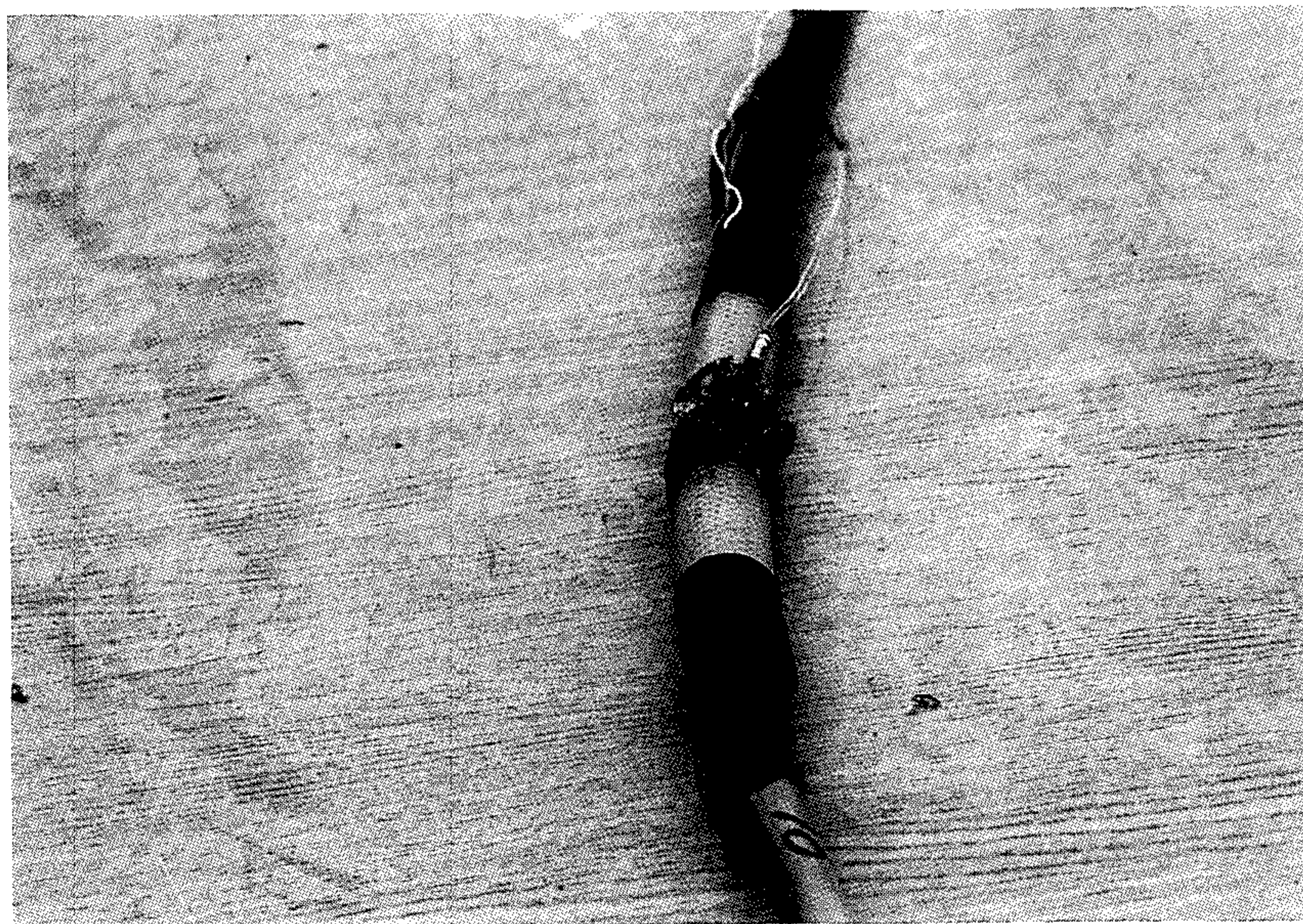
Fig. 107. Compared are the blasted detonators. Upper part: from the Hanwha detonator. Lower part: from the Nobel detonator.
