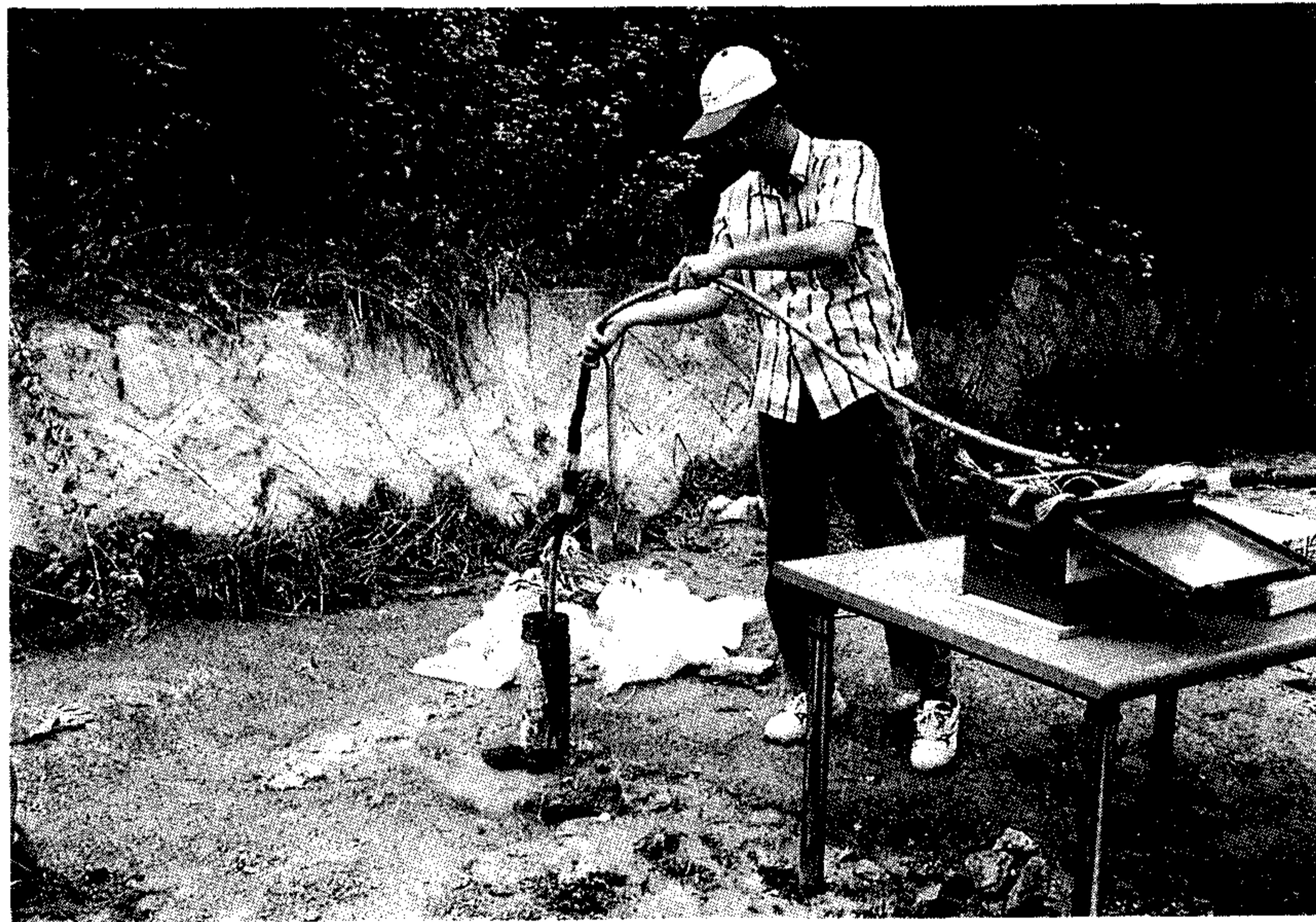
Fig. 103. Geotomographic measuring system. Shown is the operating procedure of the multiple shot borehole source.
