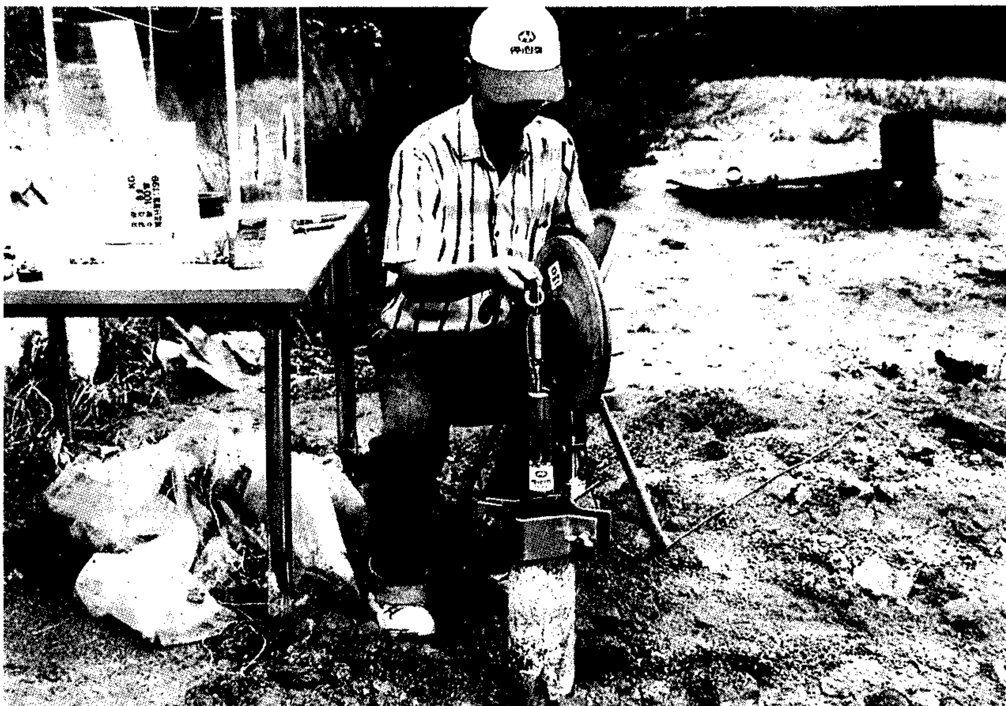
Fig. 98. Geotomographic measuring system - borehole explosive source. The picture shows the use of a single seismic detonator developed in Korea.
