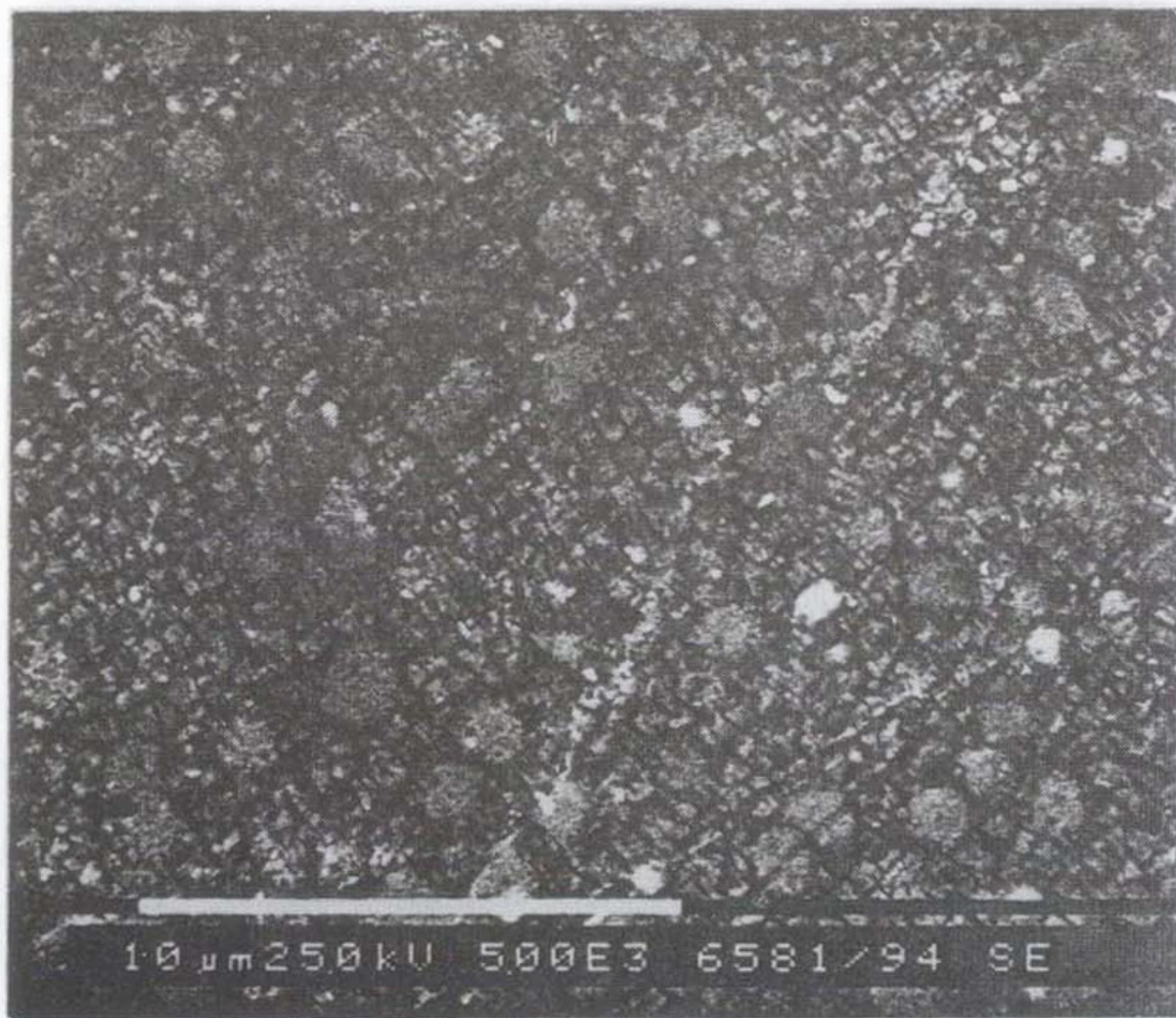
Fig. 31. Scanning Electron Micrographs after Following Gamma Prime Heat Treatment
