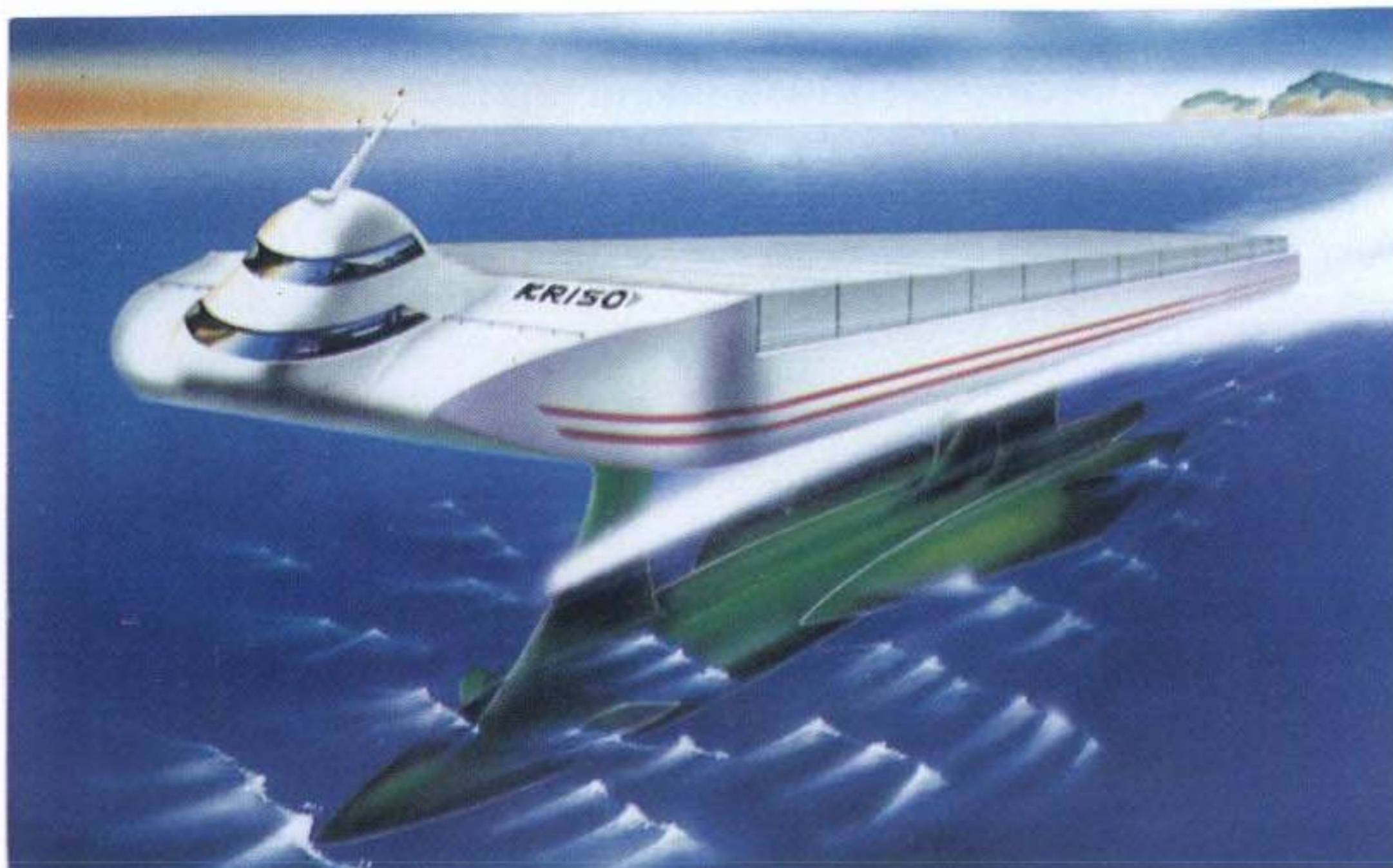
Fig. 5-18 New Hybrid Hull Form Concept (HYSWAS with Foils of Low Aspect Ratio)
