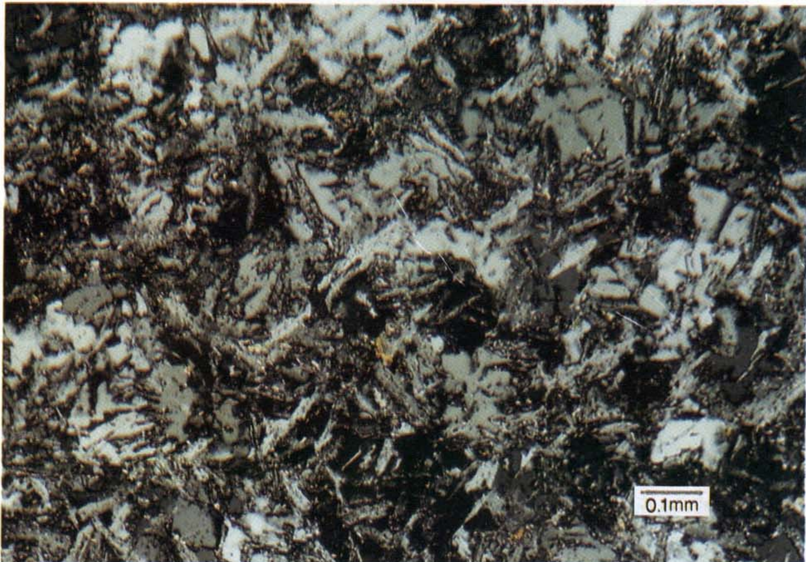
Figure 75. Micrograph of rhyolite fragment in a clayey material from Sangrari. Crossed nicols.
