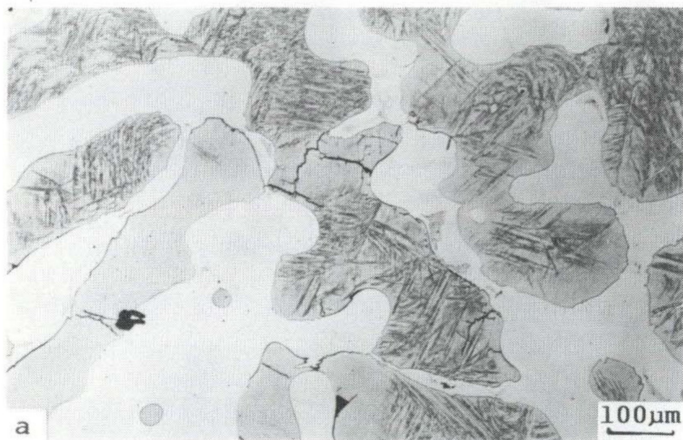
Fig.3.7 Compressive fracture and deformation mode of specimen NO.3 after heat treatment at room temperature
