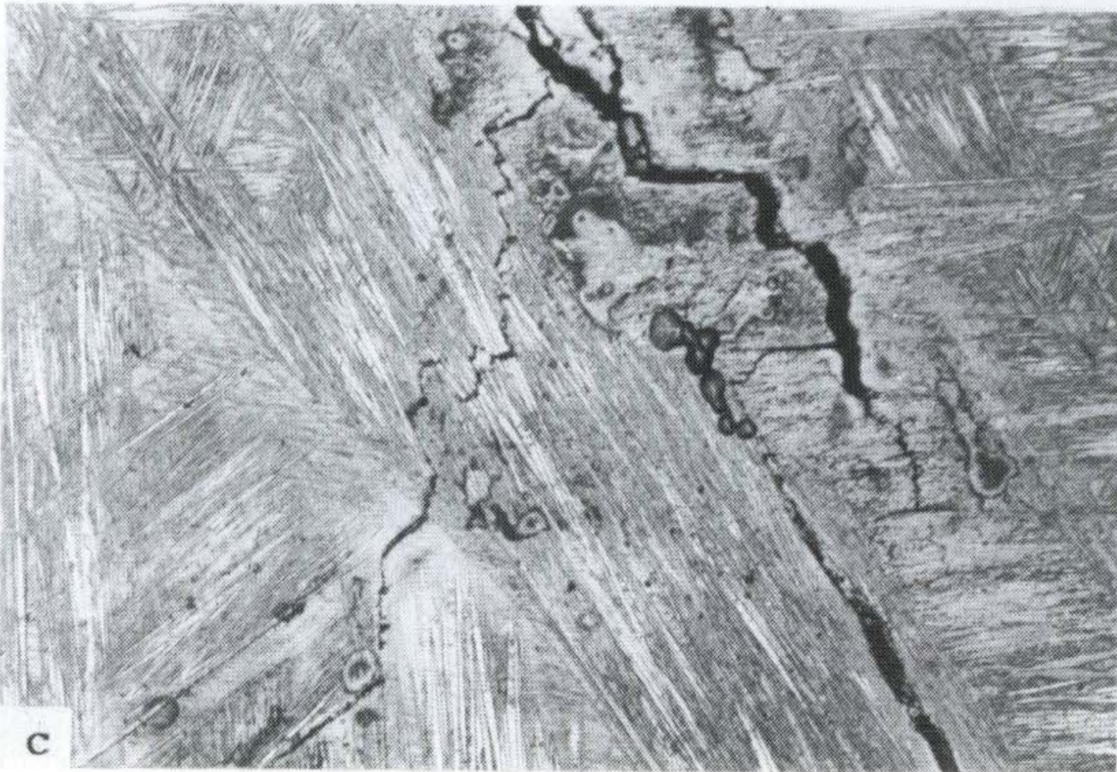
Fig. 3.9 OM micrographs showing fracture behaviour after compressive test at room temperature (a) No.1 (grain boundary crack) (b) No.2 (cracks initiated in NiAl region and propagated through interface of NiAl and Ni 3 Al) (c) No. (cleavage fracture)
