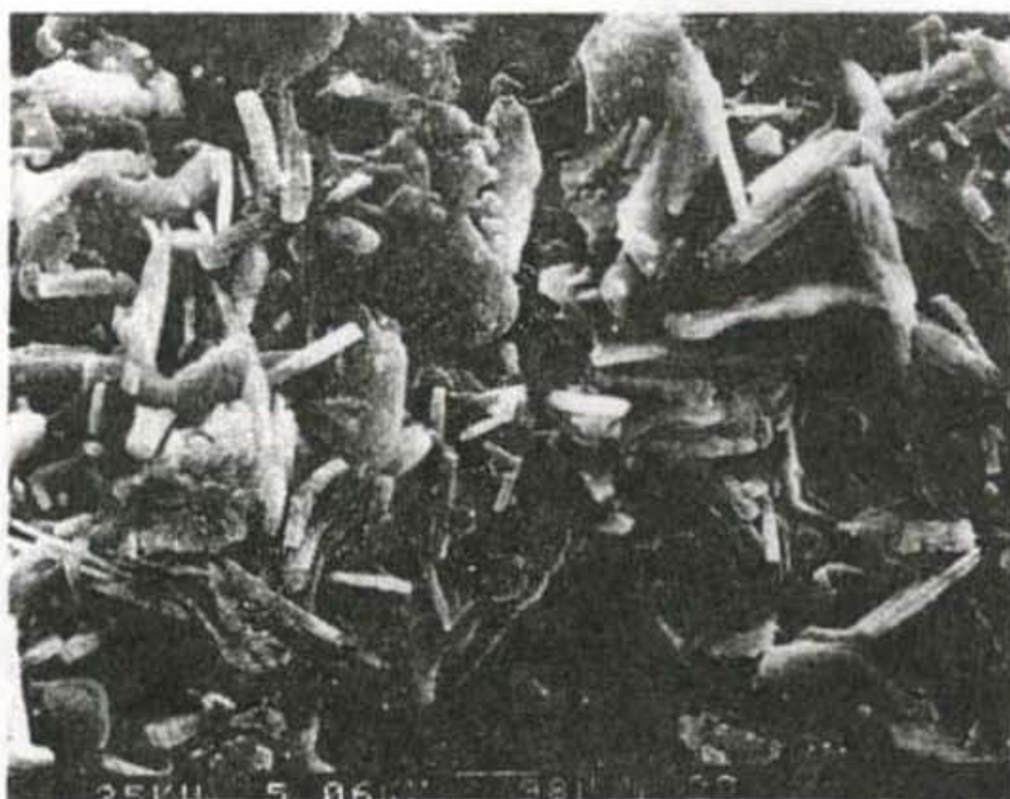
Fig. 1. Scanning electron micrograph of a spray deposited film sintered at 860°C for 10 h in air.
