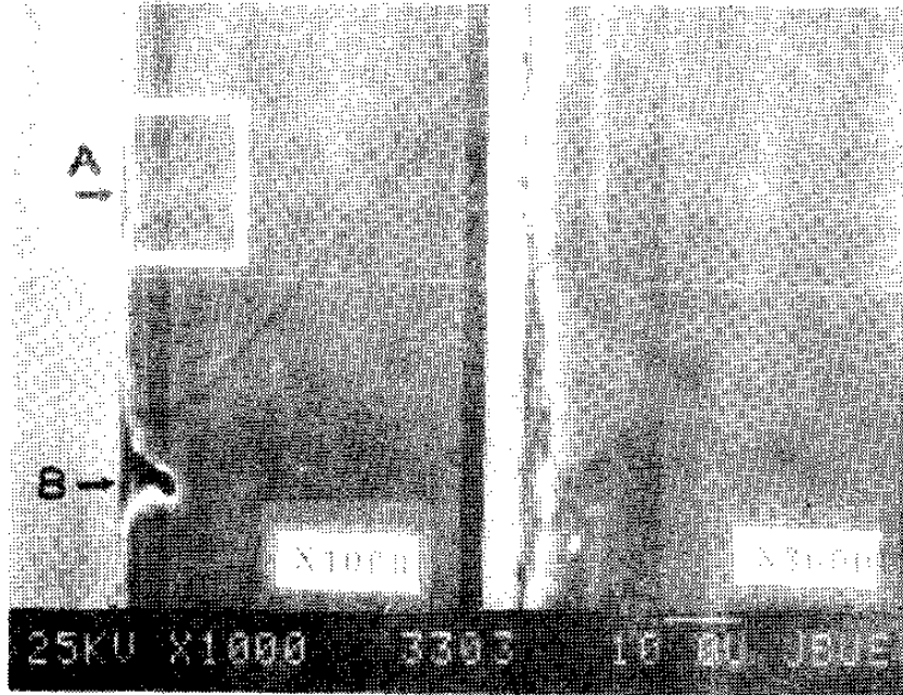
Fig.24 Photograph of the pin-hole formed in the four epitaxial layers.
